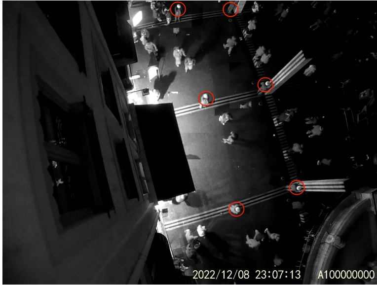
Figure 3.4: Image from camera 3 including reference points for extrinsic calibration.
