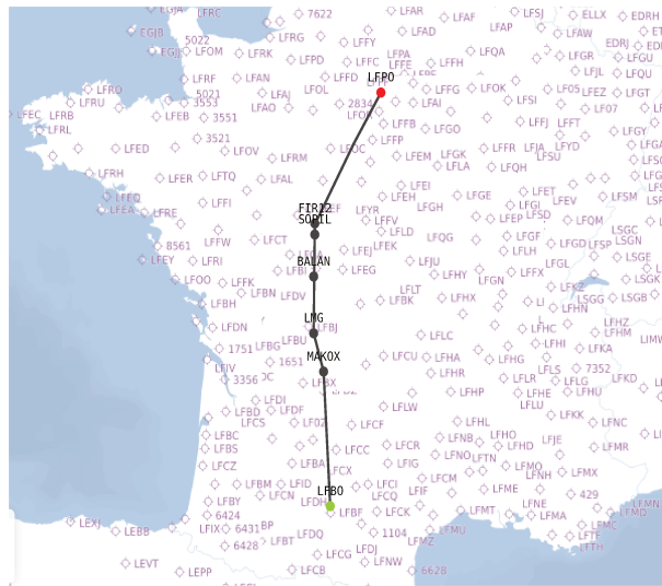
Figure 3.1: An example of a flight plan from Toulouse to Paris in France. The identification number for Toulouse airport is LFBO and the one for Paris airport is LFPO. There are several waypoints on the way from Toulouse to Paris such as MAKOX, LMG, BALAN, SOPIL FIR12 (see detail in Table 3.1).
