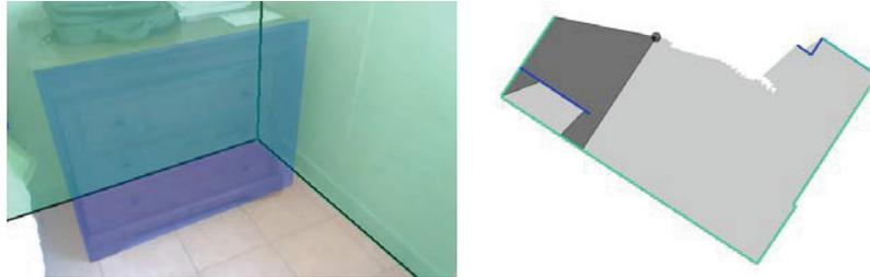
Fig. 3: Visualization of the scan progress of the scene House2. Planar patches classified as wall and clutter are represented in green and blue respectively. Intermediate colors represent intermediate probabilities. Left: augmented view of the device camera with the detected and classified planar patches. The estimated room layout is displayed with black lines. Right: visibility polygon in light gray, camera view polygon in black.
